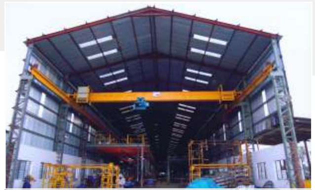
10 Ton Capacity 18 mtr. Span Single Girder EOT Crane
