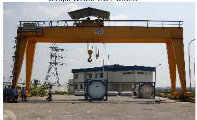
50 Ton / 10 Ton x 21 mtrs span x 12 mtrs. height Double Girder Goliath Crane
