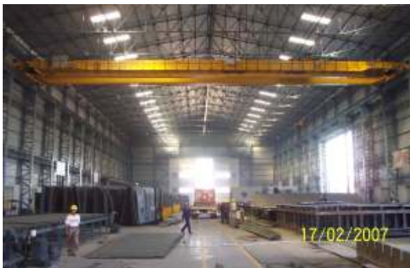
20 Ton Capacity 35 mtr. Span D/G EOT Cranes
